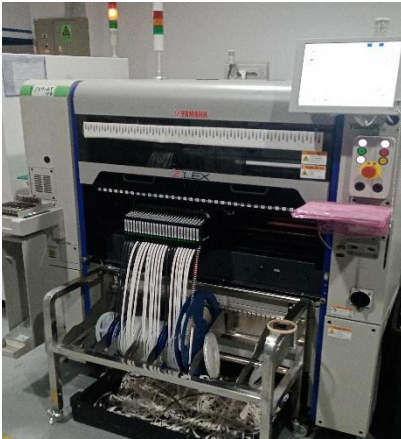
High-Speed SMT Pick-and-Place Machine YAMAHA YSM20R Component range: 0201–55 × 100 mm PCB size: 810 × 490 mm
