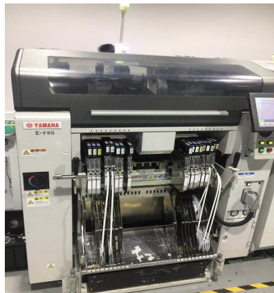
High-Speed SMT Pick-and-Place Machine YAMAHA F8S Component range: 0201–33 mm PCB size: 510 × 381 mm
