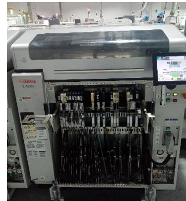
High-Speed SMT Pick-and-Place Machine YAMAHA G5S Component range: 03015–large components PCB size: 1200 × 510 mm
