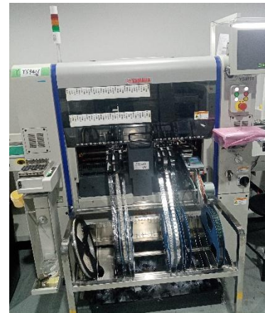
High-Speed Multi-Function Pick-and-Place Machine YAMAHA YSM10 Component range: 03015–55 × 100 mm PCB size: 510 × 460 mm
